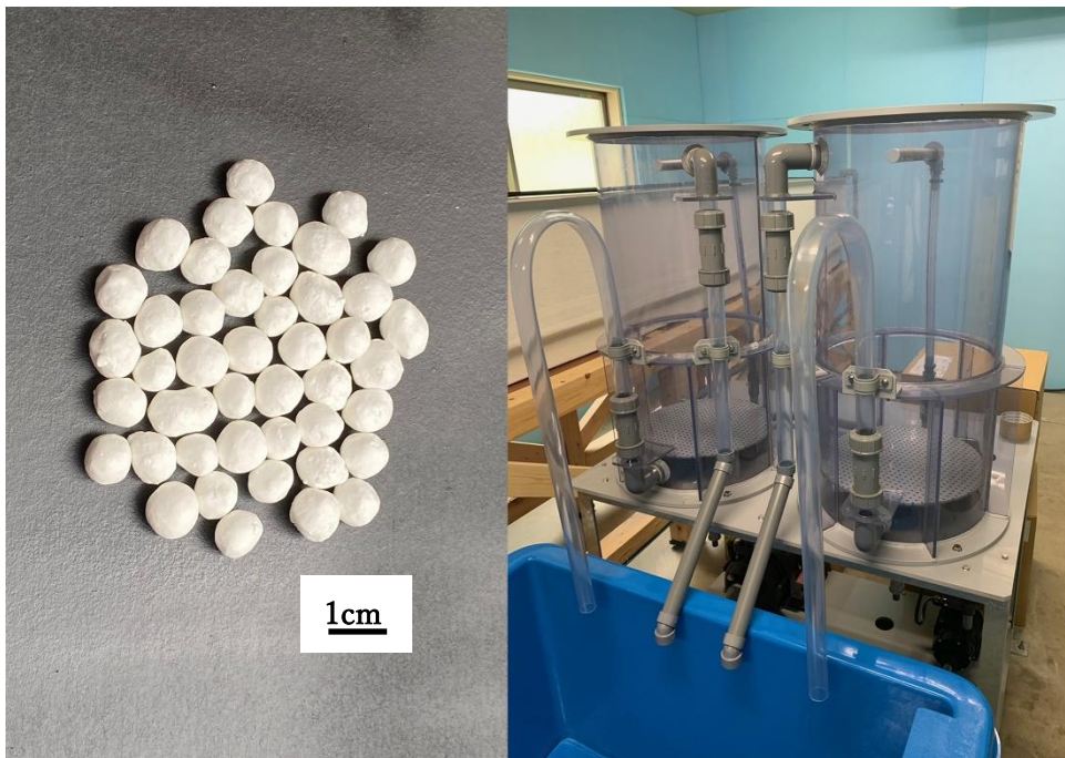
LEFT: new cellulose medium, RIGHT : Aerobic denitrification system (Copyright: Plesca Co.,Ltd.)
